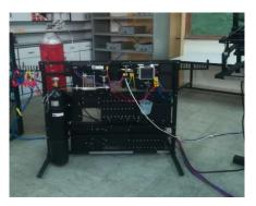
The software creates a virtual operating diagram of the facility and allows interactive monitoring and control of the system. Students may use this trainer to investigate fuel cell technology in a physical or virtual
