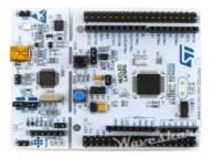
to design low-power IoT applications. To program the microcontroller it is possible to use Arduino IDE programming with C language.the most used programming is the STM32Cube Programming by use C++ languages. This tool allow the user to specifies the interfaces and peripherals that would be used in the project.
